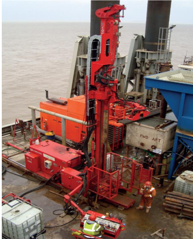
Figure 4-2: Example of a drill rig mobilised on a jack-up (Comacchio MC1200)
