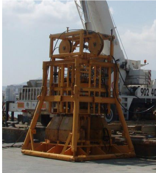
Figure 4-4: Example of a Block Push Seabed CPT System (Fugro Seacalf)
