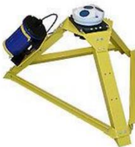
Figure 5-3: Acoustic Doppler Current Profiler (ADCP) (Wikipedia)
