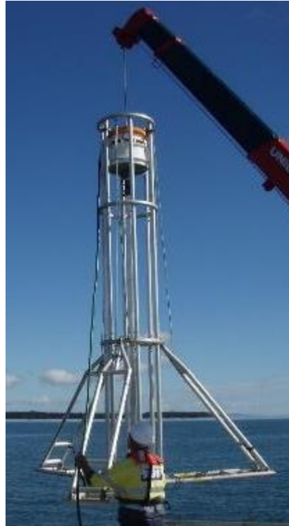
Figure 4-5: Example of a Crane Deployed Vibrocore System
