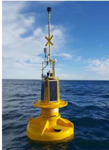
Figure 5-1: Typical Floating LiDAR (AXYS Technologies)
