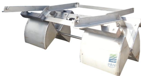
Figure 4-7: Double Van Veen Grab Sampler (OSIL)
